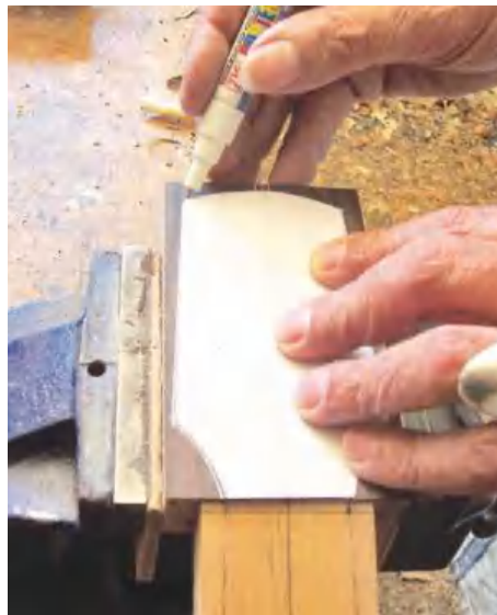
▲ Pic.25 Marking the final headstock shape out
